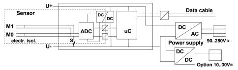
The measuring inputs are electrically isolated from the power supply by means of optocouplers. The power supply itself is also electrically isolated up to 50 V by means of the AC/DC module or the DC/DC converter (OA4390-U). The voltage at the measuring inputs themselves (between B, C, D and A or - ) must not exceed 12 volts.
