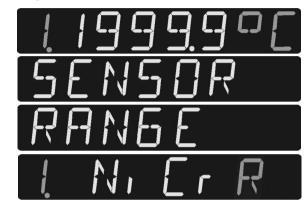
To improve the clarity of the display the channel, units, and abbreviation are slightly dimmed; channel 0 is not displayed at all.
